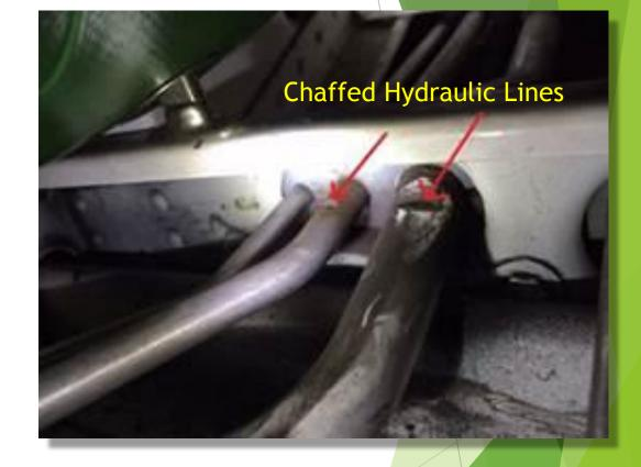
Had this tool not been found, the socket extension would have eventually chafed through the lines and depleted the main hydraulic system. Seconds from disaster?
